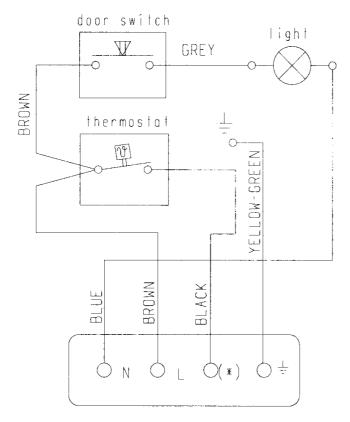
Connector \* is in the junction box market depending on producer of compressor as follows
